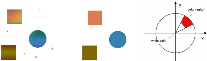
Fig. 9.22 Left. An initial image. Middle. Colours after normalization between edges. Right. A colour region in the RG-chromaticity plane
